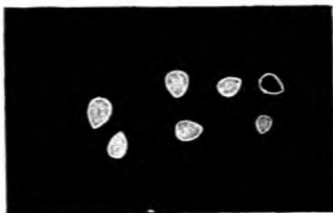
Figure 24. Contact photograph of synthetic and six natural rubies showing greater transparency of synthetic ruby to short-wave ultra-violet light
